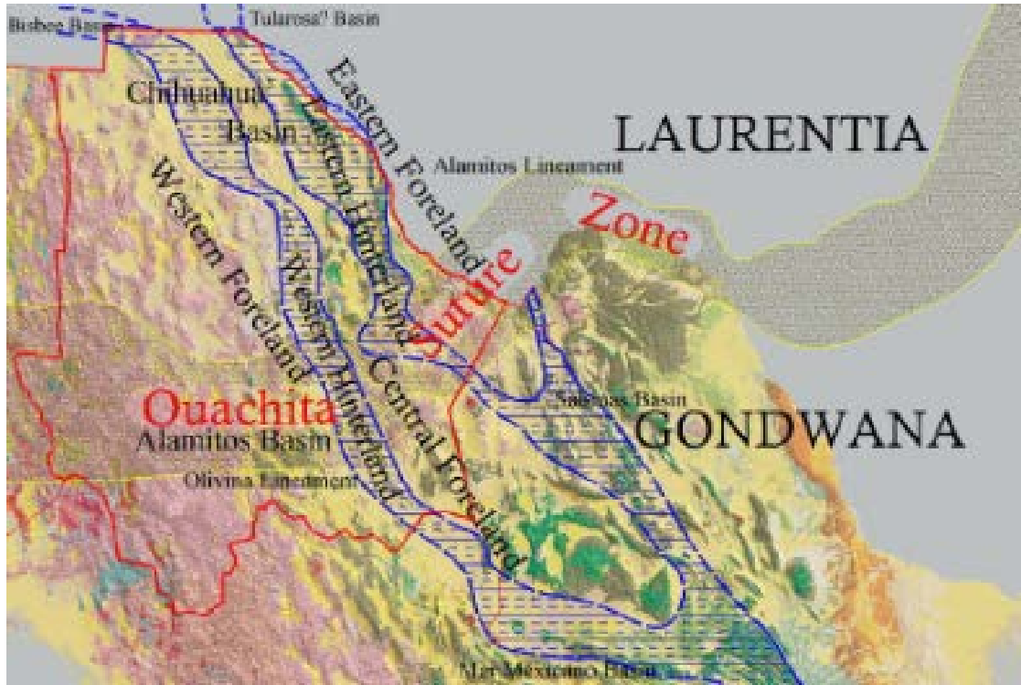
Figure 1.- Late Jurassic rift system as a tectonic model for the sedimentary basins from Chihuahua, México (Geologic base map from S.G.M., 2000)
