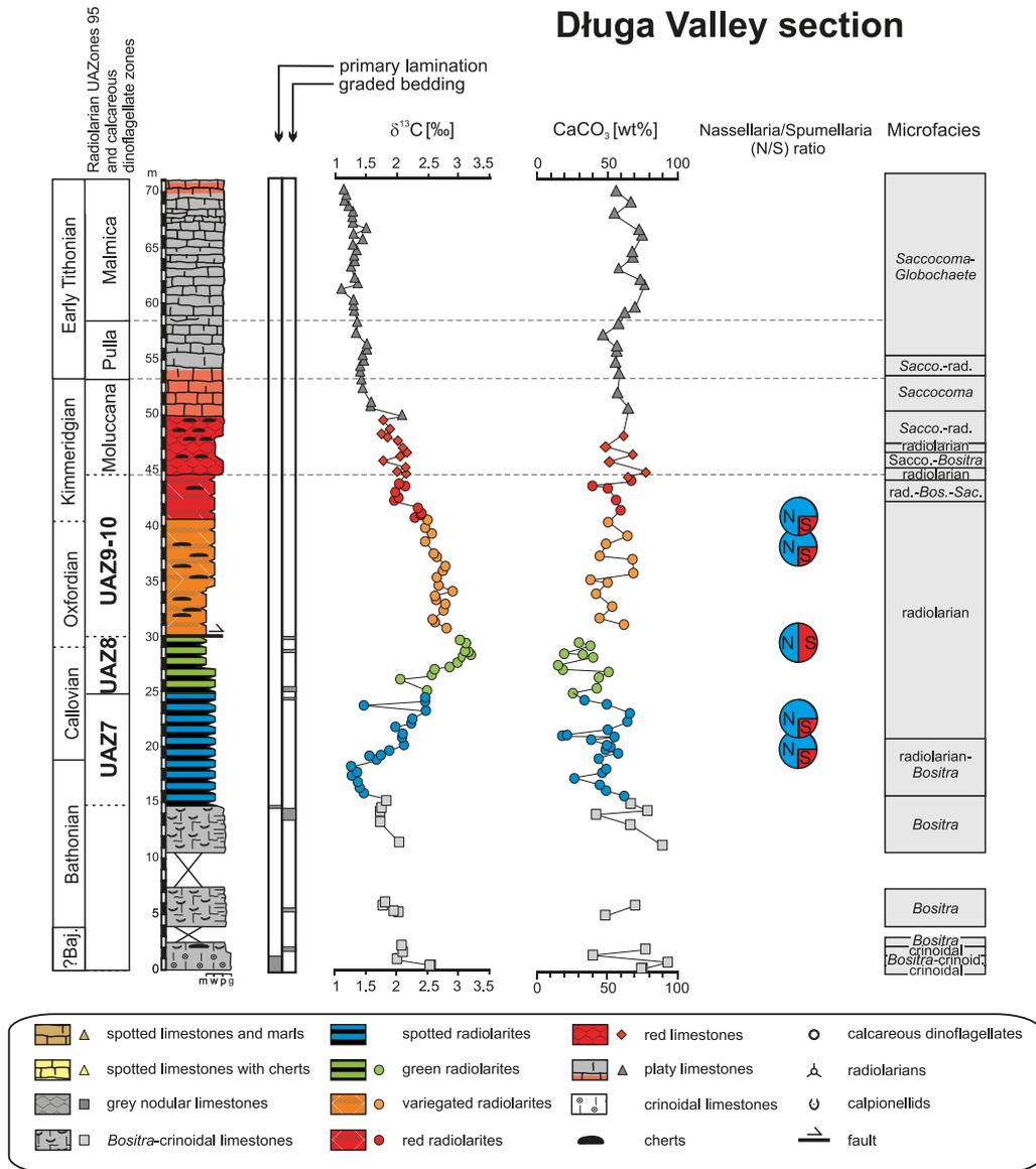
**Fig. 10.** Długa Valley section. Lithology, radiolarian and calcareous dinoflagellate biostratigraphy and results for carbon isotope measurements, CaCO<sub>3</sub> content and microfacies analysis (after Jach *et al.*, 2014; modified)
