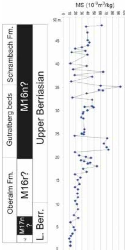
**Fig. 1.** Magnetic susceptibility (MS) record and magnetic polarity at the Oberalm/Schrambach Formation boundary
