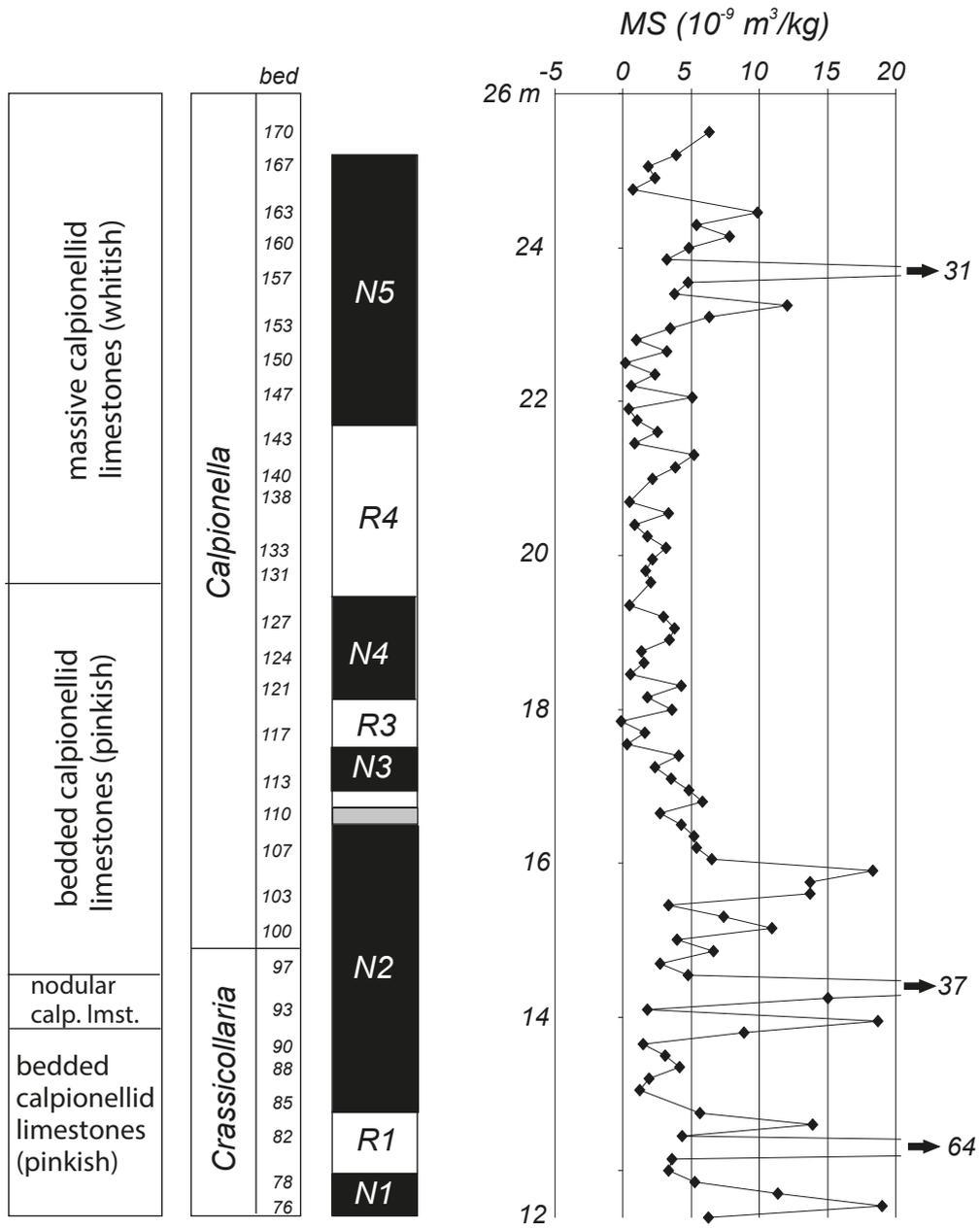
**Fig. 1.** Lithology, biostratigraphy, magnetostratigraphy and magnetic susceptibility (MS) from Veliky Kamenets section
